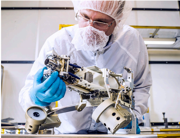
Engineer with the cryogen servicing tool (left) and the Visual Inspection Poseable Invertebrate Robot 2 (VIPIR2) (right)
